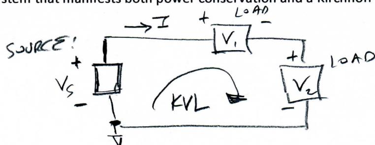
$$0 = (-V_s + V_1 + V_2)I$$
