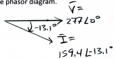
$$1\phi: \bar{S} = \bar{V} \bar{I}^* = 277 L^\circ (159.4 L + 13.1^\circ) = 43.0 \text{ kW} + 10.0 \text{ kVAR}$$
